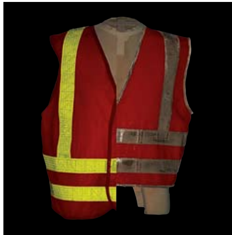
Reflectivity of Omni-Brite™ vs Glass-bead vest after 3 minutes of 1/8-inch rainfall simulation and 4 weeks of field use.
